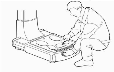
3 Check the RS-232C port of the weight scale and ankle electrode.
