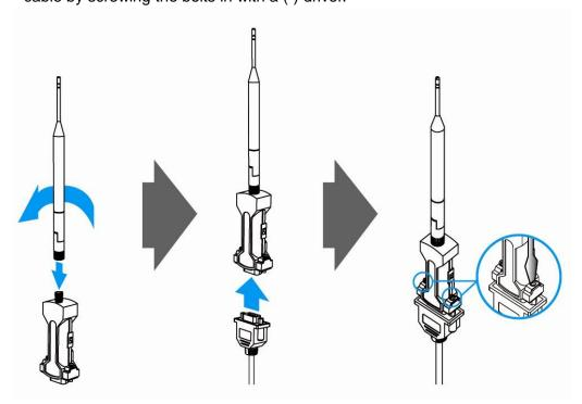
(4) Connect the unconnected side of the cable to 'EXTERNAL PORT' on the back side of the main body and then switch on the Bluetooth.
