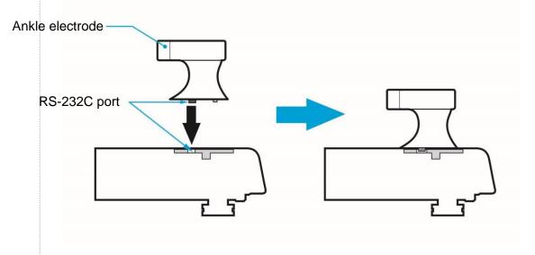
(5) Grip the ankle electrode with one hand and fix it on the scale firmly by using M12 bolt-10mm 6 angle wrench and M4 bolt-3mm 6 angle wrench.
