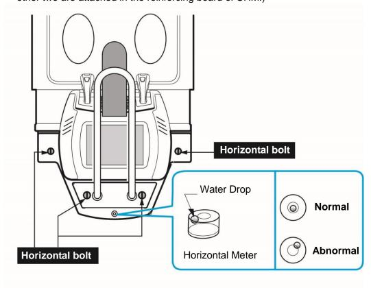
Oheck the condition after adjusting the level.
