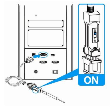
(5) Fix the Bluetooth to the back side of the main body with the provided bracket using a (+) driver. The installation is completed by turning on the device.
