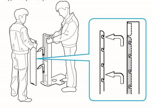
④ Fix the M6X12 wrench bolt to the groove on the bottom side of the lower body of the height using the 5mm 6angles wrench.
