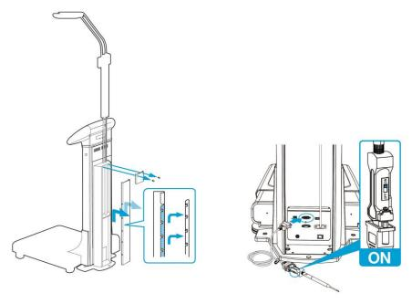
② Connect the adapter of the main body and turn it on. Push and pull down the lower cover to the arrow direction and then fix the upper cover with bolts.
