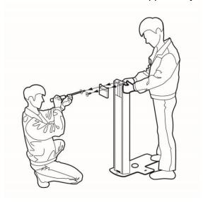
③ A person grasps the lower body not to be shaken and the other lifts up the back cover on the upper body and separate it.
