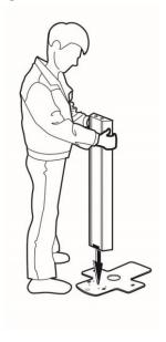
② A person grasps the lower body not to be shaken and the other unscrews two fixing bolts from the back cover on the upper body using a (+) driver and separate it.
