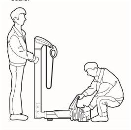
④ After connecting the scale harness and the scale PCB, stand the body up.
