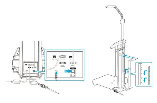
③ Check the location of the bracket hole and stick to the Bluetooth and fix it on the backside of the height meter as shown in the picture.
