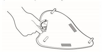
$\ensuremath{\mathfrak{B}}$  Attached the top cover on the ankle electrode to the arrow direction in the picture.
