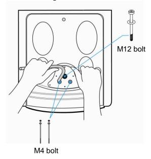
⑥ After that, try shaking the ankle electrode to check if the fixation is good or not.
