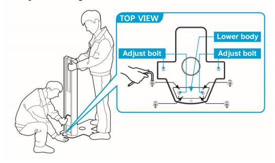
(5) While a person takes the top harness of UHM out to the inside of the lower board, the other puts a upper body supporter into two halls on the top of lower body as shown in the picture.
