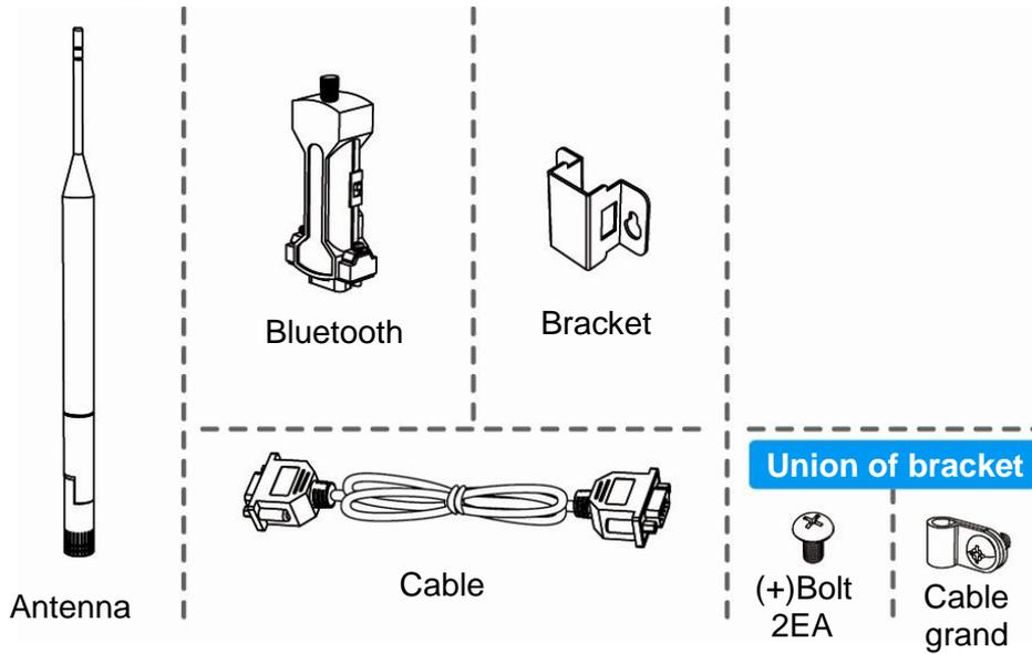
② Unscrew the (+) bolts (2EA) and cable grand (1EA) with a (+) driver. Keep the separate (+) bolts (2EA) and cable grand (1EA) to assemble a bracket and cable later.
